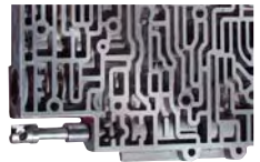
Dirty transmission valve body
